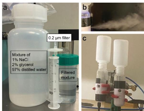
**Fig. 3** Photos of (a) the aerosol source and (b-c) artificial aerosol generators used in the STC.
