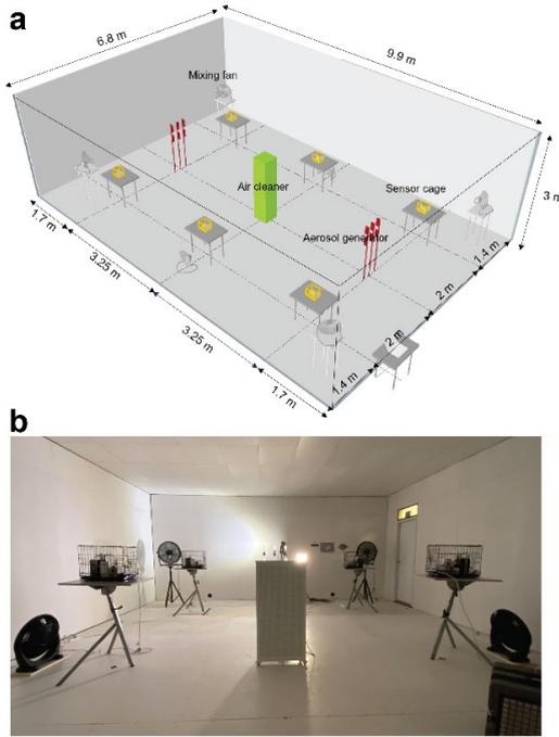
**Fig. 4.** (a) Schematic view and (b) photo of the measurement setup in the LTC. Dimensions are reported in meter.
