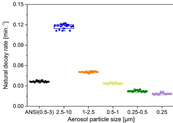
**Fig. 5.** Plots of natural decay rate of aerosols in various particle sizes from the three natural decay tests in the LTC.
