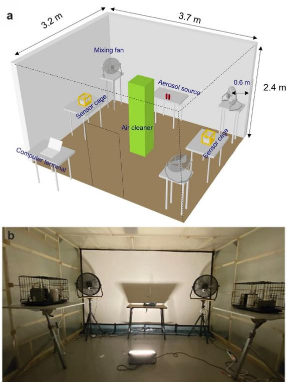
**Fig. 1.** (a) Schematic view and (b) photo of the measurement setup in the STC. Dimensions are reported in meter.
