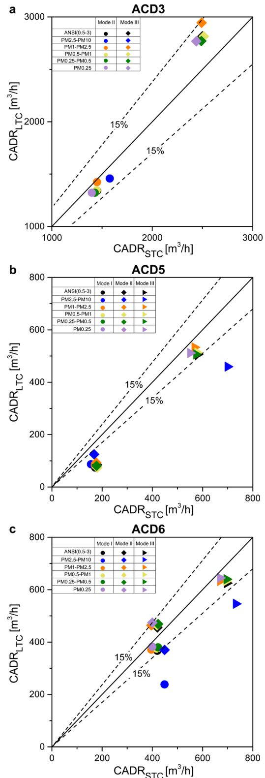
**Fig. 6.** Comparison of the CADR of (a) ACD3, (b) ACD5, and (c) ACD6 tested in STC and LTC.
